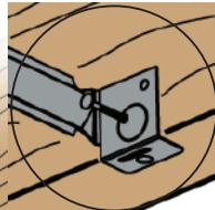
Accurate. Bottom locator tabs position the housing perfectly every time.
